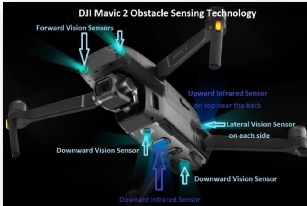
Omnidirectional Obstacle Sensing
