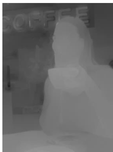
Depth Map data captured using a PDAF camera and the resulting blur map for the final image.
